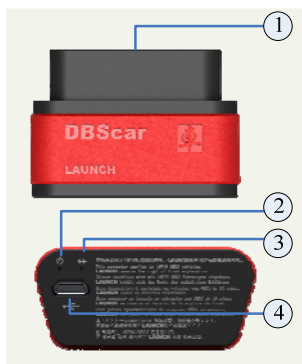
Fig. 1-5 DBScar diagnostic connector
