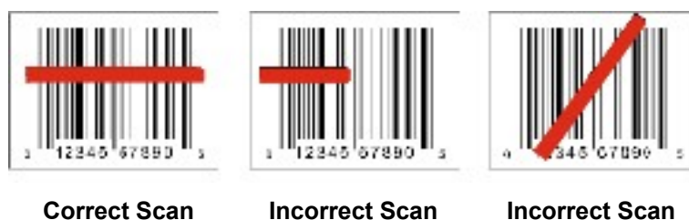
Figure 23 Laser Scanner Beam on Linear Barcode
